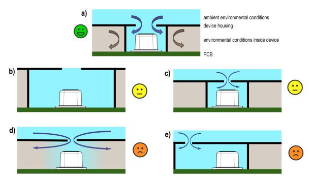
**Figure 2**: Sensor coupling to ambient environment. (a) Good coupling to the ambient air thanks to large opening in proximity to sensor and thanks to a small dead volume. (b) Moderate coupling to the ambient air due to large dead volume and (c) small opening in the device housing. (d) Poor coupling because of missing sealing from air entrapped in housing and (e) due to small opening that is far away from the sensor.
