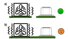
**Figure 5**: Decoupling from vibration source (side view). (a) Good decoupling is realized thanks to a gap of the support structure. (b) Bad decoupling since the PCB (green) serves as a bridge that transfers vibration to the sensor.
