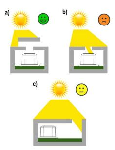
**Figure 6**: Sensor protection from sunlight (side view). (a) Good protection and (b) bad protection from incoming sunlight. (c) Good protection from sunlight, however, at the cost of bad coupling to ambient.
