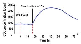
**Figure 8**: Schematic representation of the reaction time a  $CO_2$  event at t = 0s.
