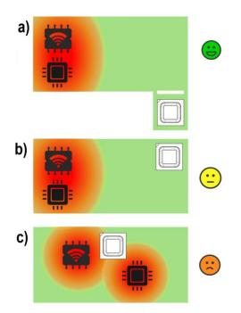
Figure 3: Sensor coupling to external heat sources (top view). The green color represents the customer PCB; the red circles indicate heat that dissipates from self-heating components. (a) Superb decoupling from external heat sources enabled by a slit in customer PCB. (c) Bad decoupling from external heat sources due to immediate proximity to self-heating components.
