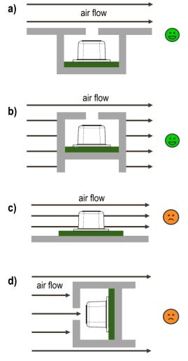
**Figure 4**: Isolation from air turbulences (side view). The grey structure represents the customer device housing. **(a-b)** Good isolation. **(c-d)** Bad isolation, as the SCD4X is exposed to wind turbulences directly.
