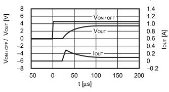
$V_{IN}$  = 4.5 V,  $C_{IN}$  =  $C_L$  = 2.2  $\mu$ F,  $C_{SS}$  = 0 nF,  $I_{OUT}$  = 1000 mA,  $V_{ON/OFF}$  = 0 V  $\rightarrow$  4.5 V,  $t_r$  = 1.0  $\mu$ s
