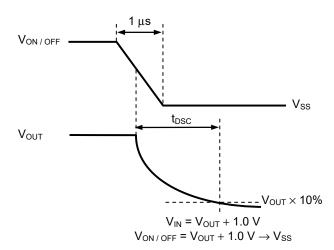
Figure 35 S-13A1 Series A / B type (with discharge shunt function)
