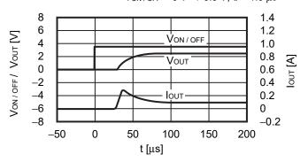
$V_{\text{IN}} = 3.5 \text{ V, } C_{\text{IN}} = C_{\text{L}} = 2.2 \text{ }\mu\text{F, } C_{\text{SS}} = 0 \text{ nF, } I_{\text{OUT}} = 1000 \text{ mA,} \\ V_{\text{ON}/\text{OFF}} = 0 \text{ V} \rightarrow 3.5 \text{ V, } t_{\text{r}} = 1.0 \text{ }\mu\text{s} \\$
