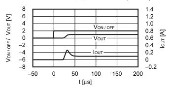
$V_{IN}$  = 2.0 V,  $C_{IN}$  =  $C_L$  = 2.2  $\mu$ F,  $C_{SS}$  = 0 nF,  $I_{OUT}$  = 1000 mA,  $V_{ON/OFF}$  = 0 V  $\rightarrow$  2.0 V,  $t_r$  = 1.0  $\mu$ s
