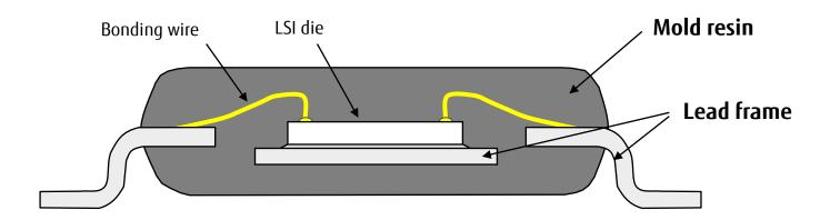
Lead frames and mold resins are the main materials for packaging components, which will no longer be procurable in March 2022 due to the end of material production at component manufacturers.
