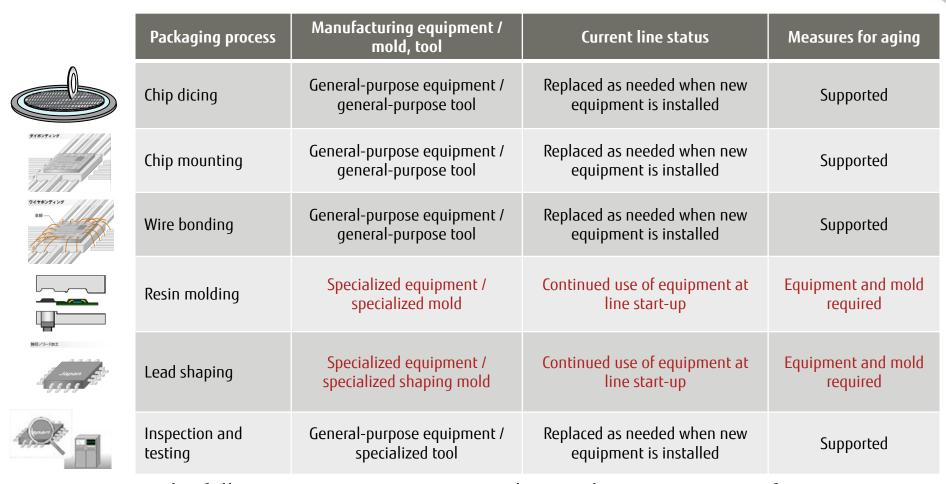
\*The following equipment is required to implement measures for aging production lines.
