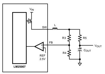
Figure 6. Low Ripple Output Configuration
