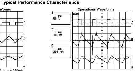
LM25007 Operation:  $V_{OUT}$  = 10V,  $V_{IN}$  = 42V,  $I_{OUT}$  = 250mA CH1: Switch Node, CH2:  $V_{OUT}$  (AC), CH4: Inductor Current Figure 2.
