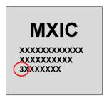
3)Package Label outside of shipping box can also identify the wafer Fabs. Lot# can be identified on the label. Lot# starts with number "2, 3, or 5" means the device is from Fab 2, whereas Lot# starts with number "7,8, or 9" means the device is from Fab 5.
