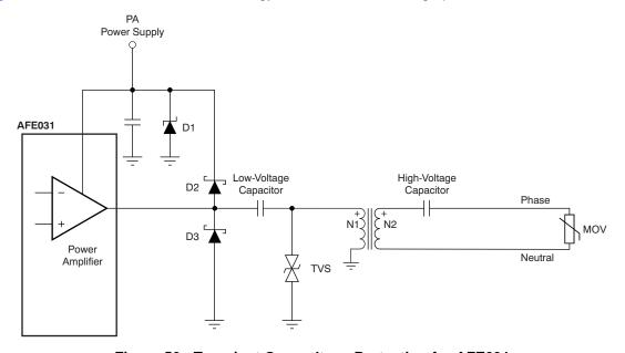
Figure 50. Transient Overvoltage Protection for AFE031
