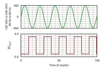
Figure 38. Non-Isolated Zero Crossing Waveforms
