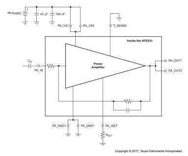
Figure 25. Typical Connections to the PA
