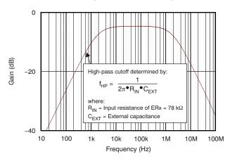
Figure 42. ERx Block Frequency Response
