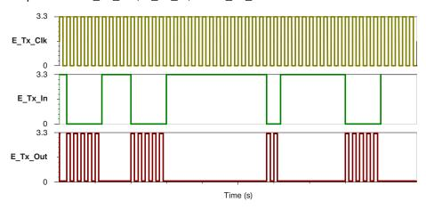
Figure 41. ETx Block Transfer Function
