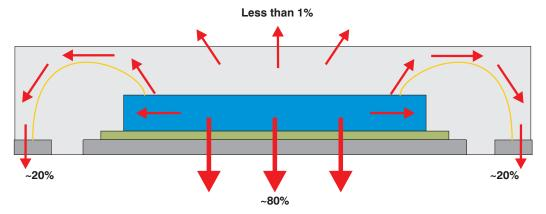
Figure 52. Heat Flow in the QFN Package
