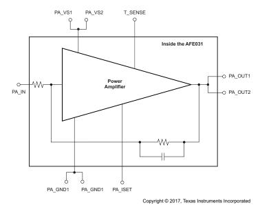
Figure 24. PA Block Equivalent Circuit
