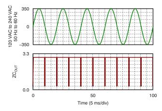
Figure 40. Isolated Zero Crossing Waveforms
