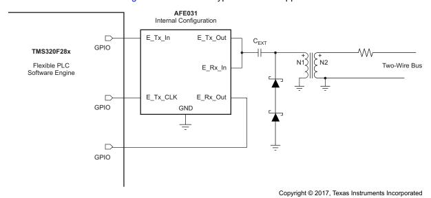
Figure 43. Typical Two-Wire Application for ETx and ERx
