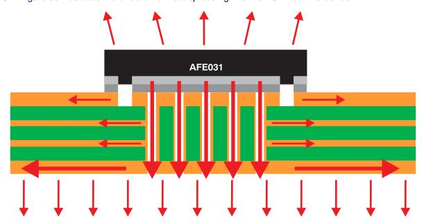
Figure 53. Heat Spreading into PCB
