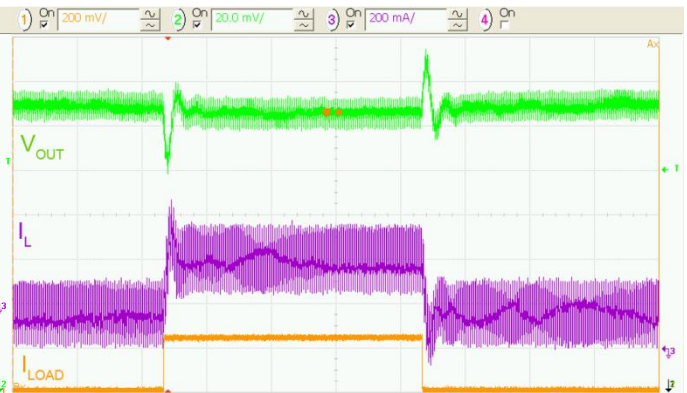
Figure 29. Load Transient 150 to 400 mA, 3.6 V_{IN}
