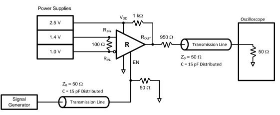
Figure 8. Receiver TRI-STATE Delay Test Circuit
