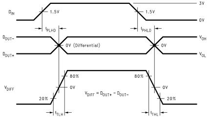
Figure 3. Driver Propagation Delay and Transition Time Waveforms
