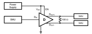
Figure 1. Driver  $V_{\text{OD}}$  and  $V_{\text{OS}}$  Test Circuit
