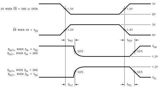
Figure 5. Driver TRI-STATE Delay Waveform
