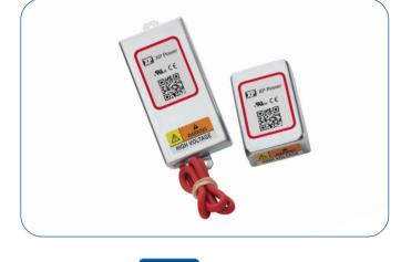
The C Series is a line of miniature, regulated high voltage power supplies. Each model is programmed from 0 to 100% of rated output via a 0 to +5 volt, DAC-compatible, high-impedance programming input voltage. An externally accessible potentiometer provides adjustable gain trim, allowing for individual calibration of units.
