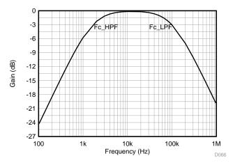
Figure 95. CW Summing Amplifier Transfer Function
