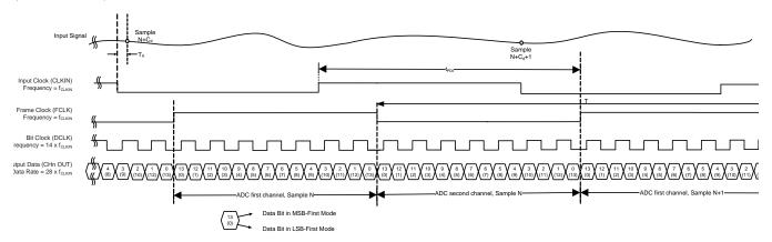
Figure 80. 14-Bit, 2X Data Rate Output Timing Specification
