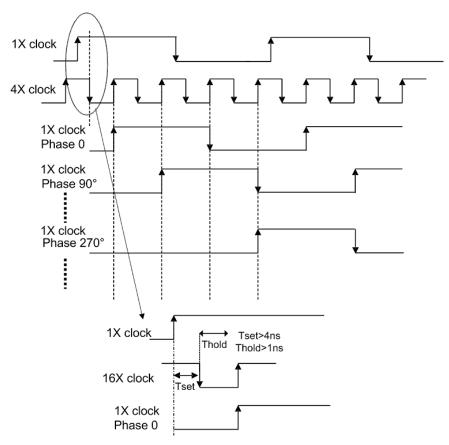
Figure 92. 8 ×  $f_{cw}$  and 4 ×  $f_{cw}$  Timing Diagram
