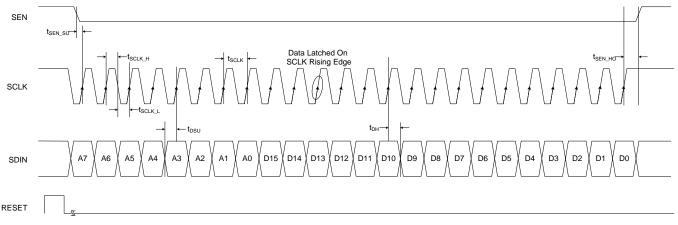
Figure 101. Serial Interface Timing Diagram
