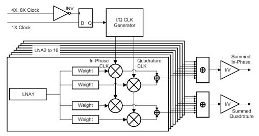
Figure 91. 8 ×  $f_{cw}$  and 4 ×  $f_{cw}$  Block Diagram
