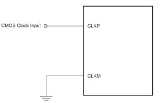
Figure 72. Single-Ended Clock Driving Circuit
