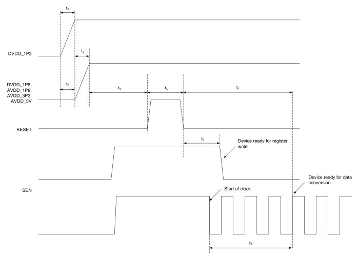
NOTE: 10  $\mu$ s < t<sub>1</sub> < 50 ms, 10  $\mu$ s < t<sub>2</sub> < 50 ms, t<sub>3</sub> > t<sub>1</sub>, t<sub>4</sub> > 10 ms, t<sub>5</sub> > 100 ns, t<sub>6</sub> > 100 ns, t<sub>7</sub> > 4 ADC clock cycles, and t<sub>8</sub> > 100  $\mu$ s.
