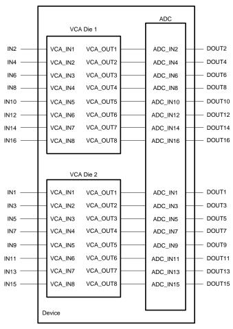
Figure 114. Channel Mapping: VCA Dies
