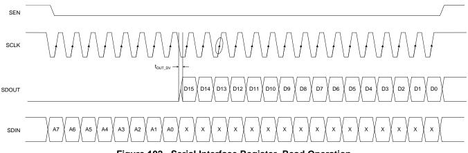
Figure 102. Serial Interface Register, Read Operation
