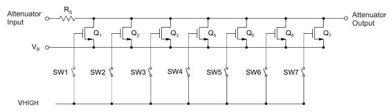
Figure 67. Simplified Voltage-Controlled Attenuator (Digital Structure)
