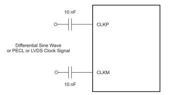
Figure 73. Differential Clock Driving Circuit
