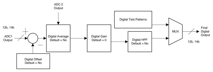
Figure 82. ADC Digital Block Diagram
