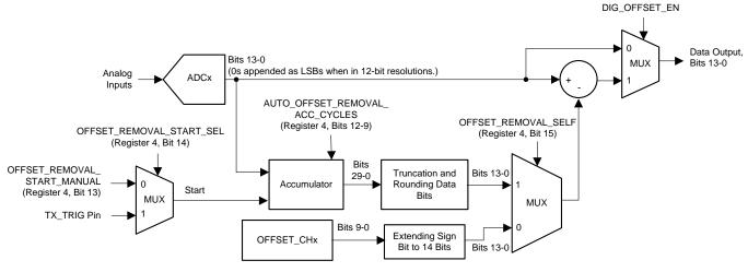
Figure 83. Digital Offset Correction Block Diagram
