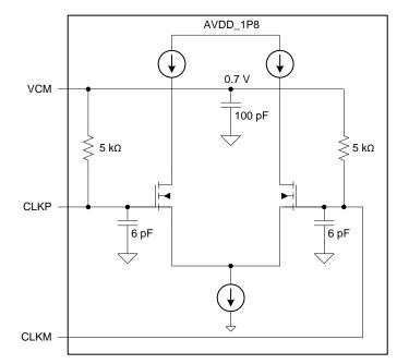
Figure 71. Internal Clock Buffer for Differential Clock Mode
