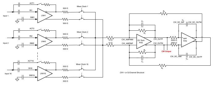
Figure 94. CW Summing Amplifier and High-Pass Filter Implementation
