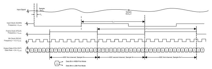
Figure 81. 12-Bit, 2X Data Rate Output Timing Specification
