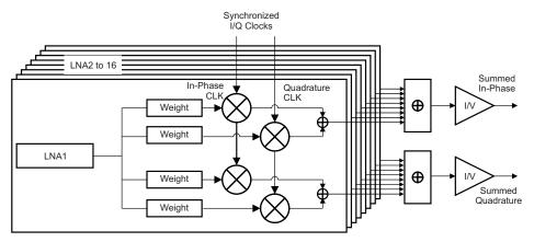
Figure 93. 1 ×  $f_{cw}$  Mode Block Diagram
