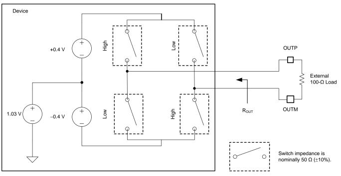
Figure 76. LVDS Output Circuit
