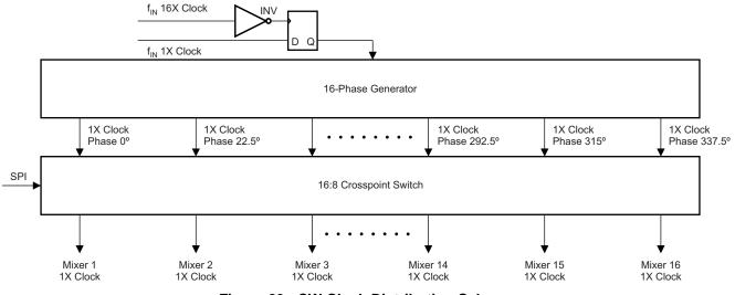
Figure 89. CW Clock Distribution Scheme
