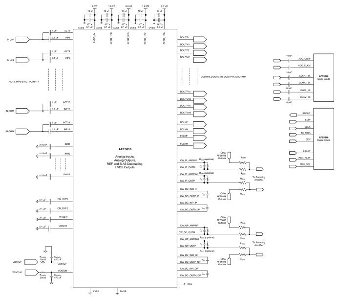
(1) N represents the number of capacitors connected to the supply. Placing at least one capacitor for every three supply pins is recommended.
