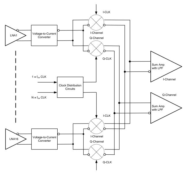
Figure 86. Simplified Block Diagram of the CW Path
