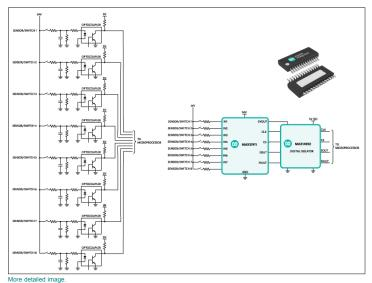
More detailed image. Figure 7. A32-channel PLC I/O module integrates an 8-to-1 digital-input serializer (MAX31911) with an integrated digital isolator (MAX14932) to reduce part count by 70% and lowers Figure 7. A32-channe solution size by 63%.
