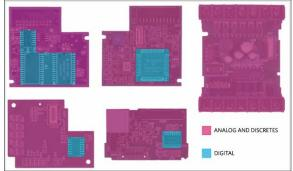
Figure 6. The system integration challenge in MicroPLCs is evident here where analog and digital components are visible on system boards.
