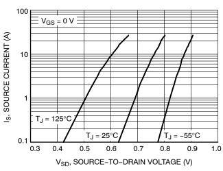
Figure 10. Diode Forward Voltage vs. Current
