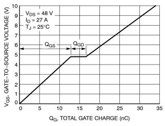
Figure 8. Gate-to-Source vs. Total Charge
