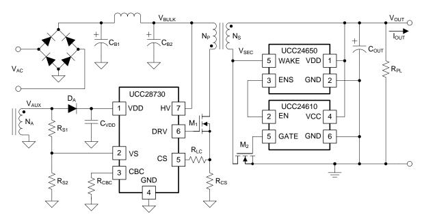
Figure 20. Simplified Application With Ground-Referenced Synchronous Rectifier
