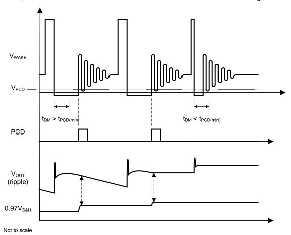
Figure 11. Timing Diagram of Internal PCD Signal
