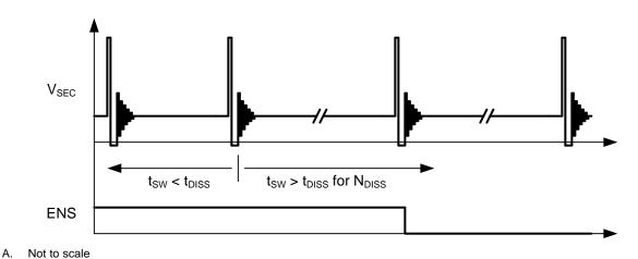
Figure 18. Simplified Timing Diagram of ENS Behavior for Gradual Decrease of Load
