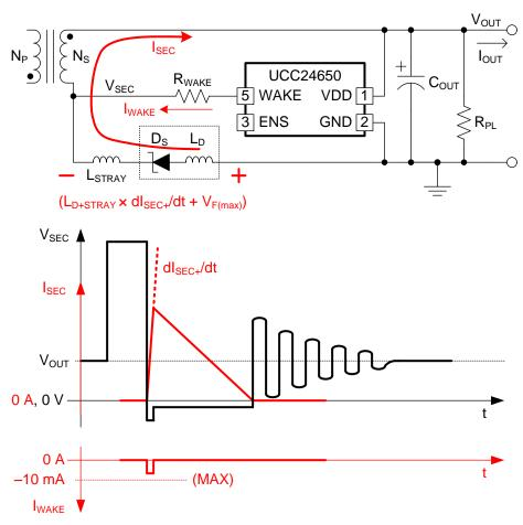
Figure 16. High dl<sub>SEC</sub>/dt may Generate Significant I<sub>WAKE</sub>.
