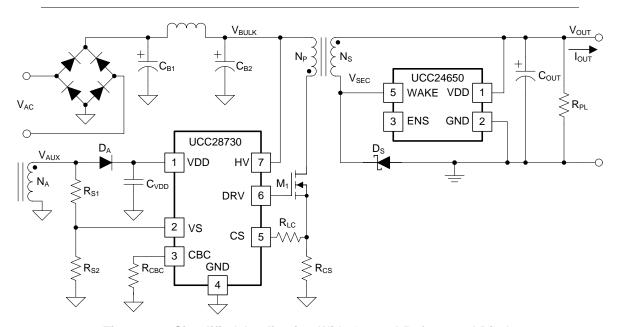
Figure 19. Simplified Application With Ground-Referenced Diode
