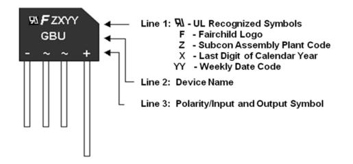
Reason for Change: To reflect UL certification on package surface marking.
