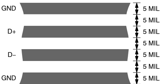
Figure 22. Typical Arrangement of Signal Tracks
