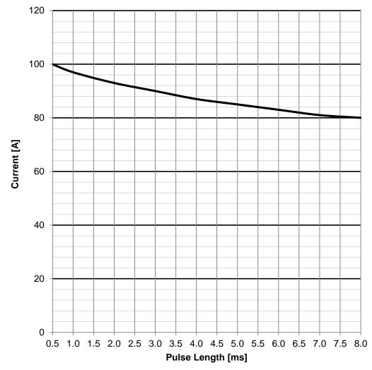
valid for ambient temperature: +25°C; 8 ms pulse length, single pulse
