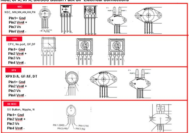
**NSC, SX, SCC DIP Electrical Connections**
