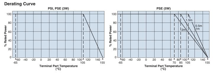
For resistors operated at a terminal part temperature of described for each size or above, a power rating shall be derated in accordance with the derating curve. Please refer to "Introduction of the derating curve based on the terminal part temperature" in the beginning of our catalog before use.
