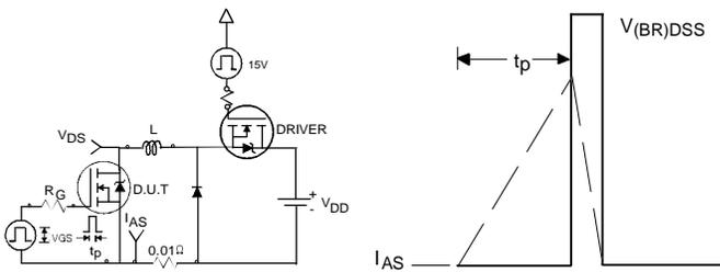
**Fig 14.** Unclamped Inductive Test Circuit and Waveform
