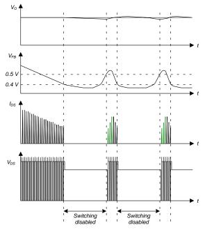
Figure 29. Burst Mode Operation
