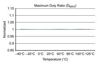
Figure 16. Maximum Duty Ratio (D<sub>MAX</sub>) vs. T<sub>A</sub>
