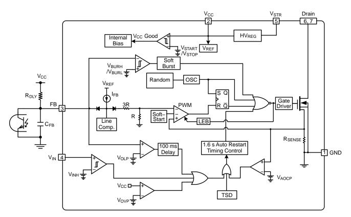
Figure 2. Internal Block Diagram
