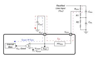
Figure 17. Startup and HV<sub>REG</sub> Block
