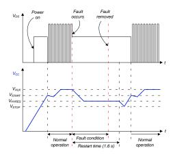
Figure 19. Auto–Restart Protection Waveforms
