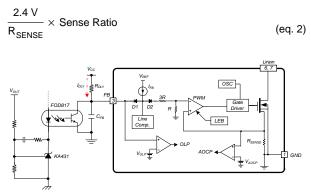
Figure 18. Pulse Width Modulation Circuit
