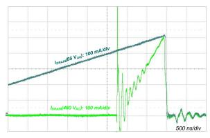
Figure 30. I<sub>LIMIT</sub> Waveforms (85 V<sub>AC</sub> vs. 460 V<sub>AC</sub>)
