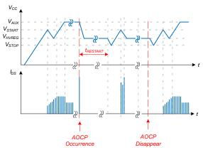
Figure 22. AOCP Waveforms
