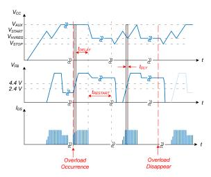
Figure 20. OLP Waveforms
