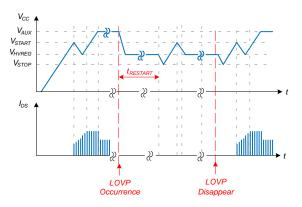
Figure 25. LOVP Waveforms
