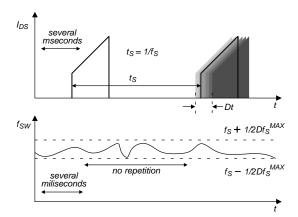
Figure 27. Frequency Fluctuation Waveforms
