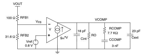
Figure 34. Example of the Feedback Compensation Network
