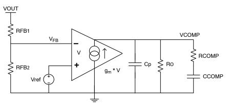
Figure 32. Feedback Compensator Network Model
