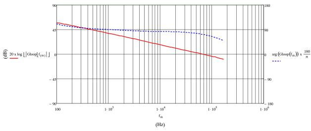
Figure 36. Bode Plot of the Total Loop
