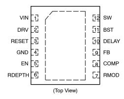
Figure 3. Pin Connections
