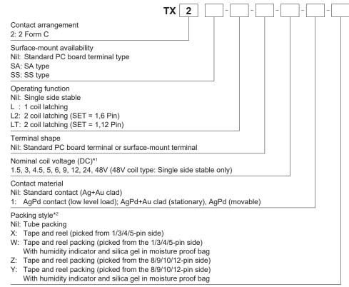
Note 1) In case of 5 V transistor drive circuit, it is recommended to use 4.5 V type relay
