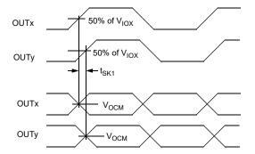
Figure 34. Output Enable/Disable/Frequency Select Timing
