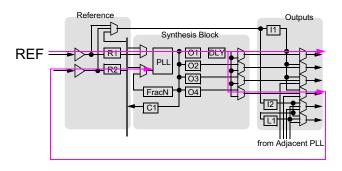
The CY27410 provides the frequency-multiplying ZDB by modulating the R1 and R2 values in the integer ratio. If both the values are identical, the CY27410 acts as a simple ZDB.
