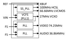
Apart from having the audio and video clocks following the 27-MHz VCXO input, they also need complex divider ratios to generate the output frequencies. Commonly used divider ratios for audio and video signals are listed in Table 1.
