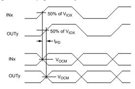
Figure 35. HCSL Single-ended Measurement Point-2
