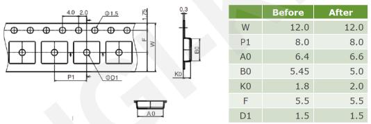
There is no change in the tape width, pitch, hole diameter, or hole position. The dimensions of the pocket are different.
