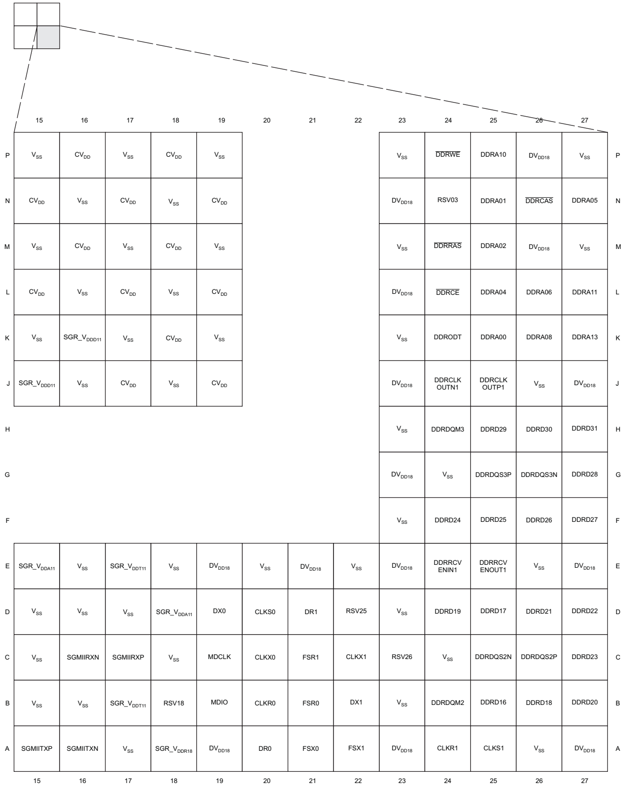
Figure 2-4. C6474 Pin Map (Bottom View) [Quadrant C]
