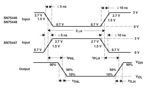
NOTES: A. The pulse generator has the following characteristics: PRR = 100 kHz,  $Z_O = 50 \Omega$ .
