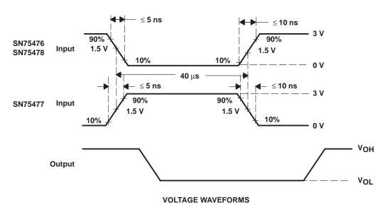
NOTES: A. The pulse generator has the following characteristics: PRR = 12.5 kHz,  $Z_O = 50 \Omega$ .
