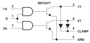
Positive Logic:  $Y = \overline{AS}$  or  $\overline{A} + \overline{S}$
