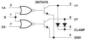
Positive Logic: Y = A+S or  $\overline{A} \overline{S}$
