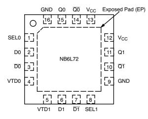
Figure 2. Pin Configuration (Top View)
