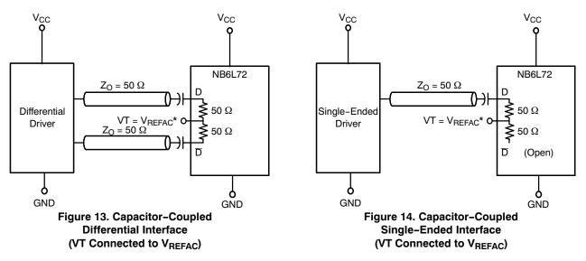
$^{*}V_{\text{REFAC}}$  bypassed to ground with a 0.01  $\mu\text{F}$  capacitor
