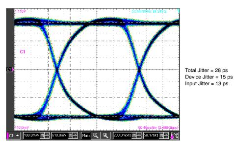
Figure 18. Typical Output Wave Form – Data Signal PRBS 2<sup>23</sup>–1 Room Temperature, 75 mV Input Amplitude, 3 Gb/s (X-scale = 80 ps/DIV; y-Scale = 100 mV/DIV)
