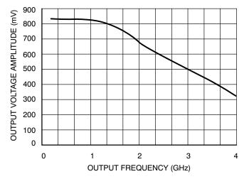
Figure 16. Output Voltage Amplitude (V<sub>OUTPP</sub>) versus Output Frequency at Ambient Temperature (Typical)
