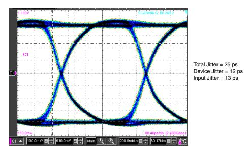
Figure 17. Typical Output Wave Form – Data Signal PRBS 2<sup>23</sup>–1 Room Temperature, 400 mV Input Amplitude, V<sub>CC</sub> = 2.5 V, 2.488 Gb/s (X-scale = 80 ps/DIV; y-Scale = 100 mV/DIV)
