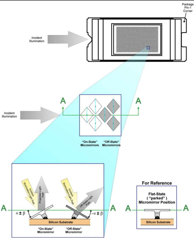
Figure 8-2. Micromirror Landed Positions and Light Paths
