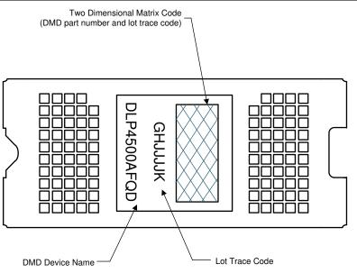
Figure 12-3. Device Markings for FQD
