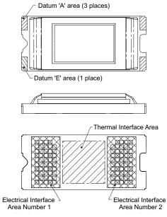
Figure 7-4. System Interface Loads for FQD
