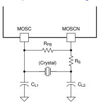
C<sub>L</sub> = crystal load capacitance in F
