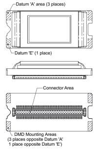
Figure 7-3. System Interface Loads for FQE
