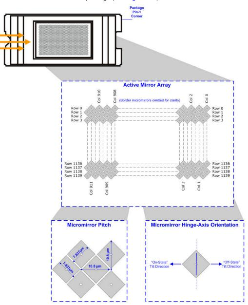
Figure 8-1. Micromirror Array, Pitch, and Hinge-Axis Orientation
