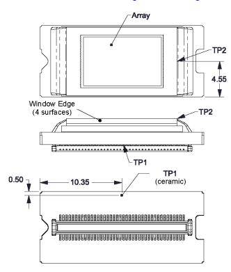
Figure 8-3. Thermal Test Point Location - FQE Package
