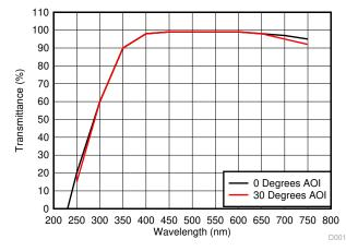
Figure 7-6. DLP4500 DMD Window Transmittance
