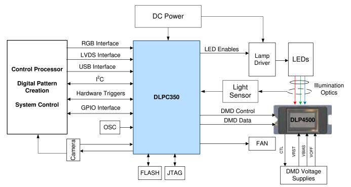
Figure 9-1. Typical Application Schematic
