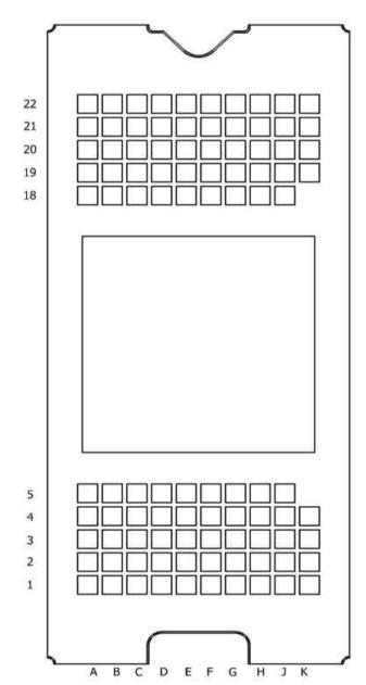
Figure 6-2. FQD Package LCCC (98) Bottom View
