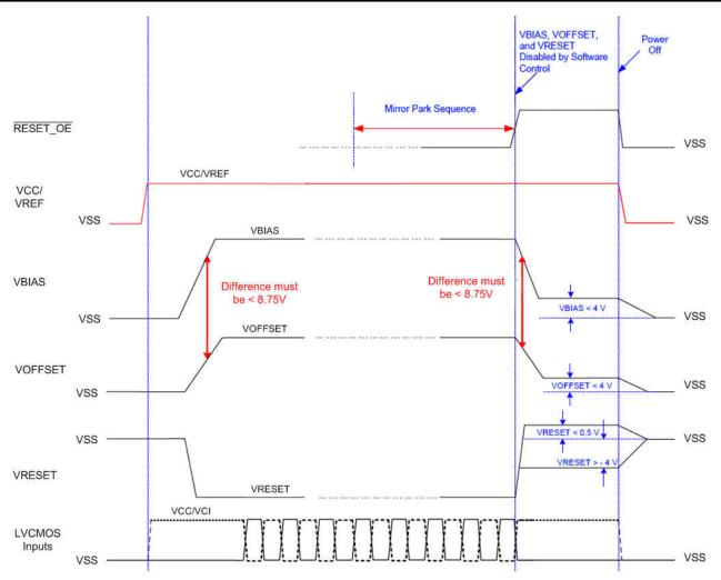
Figure 10-1. Power-Up and Power-Down Timing
