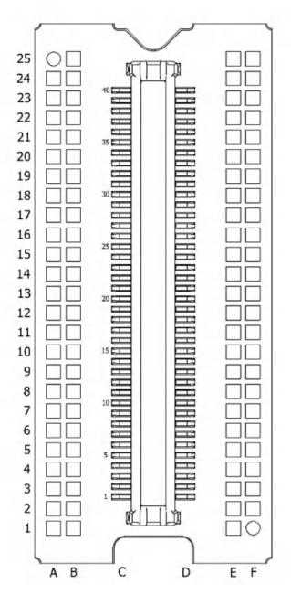
Figure 6-1. FQE Package. LCCC (80). Bottom View.
