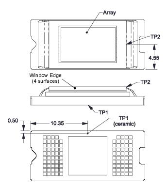
Figure 8-4. Thermal Test Point Location - FQD Package
