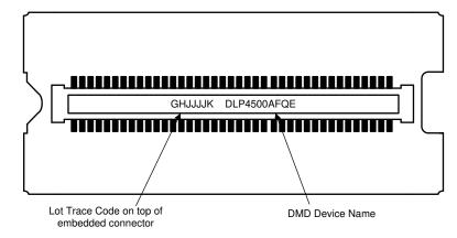
Figure 12-2. Device Marking for FQE
