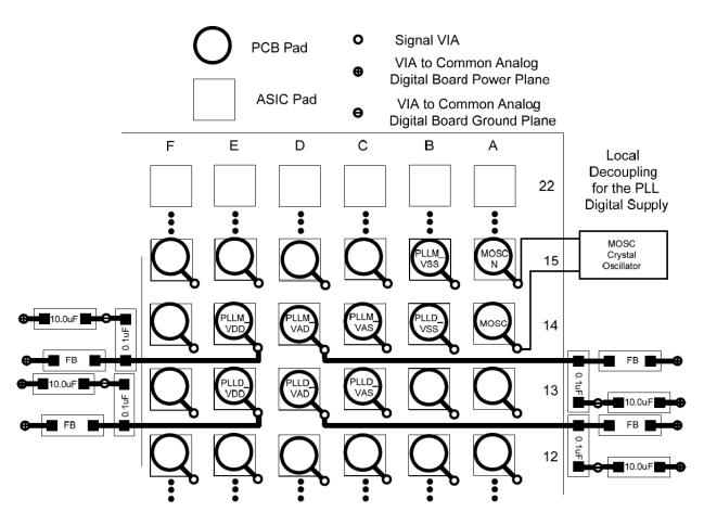
Figure 11-4. PLL Filter Layout
