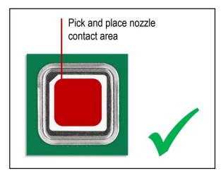
SCD4x P&P nozzle contact area. The edge in the protection membrane serves as a polarity mark indicating the pin 1 mark on the backside of the PCB.
