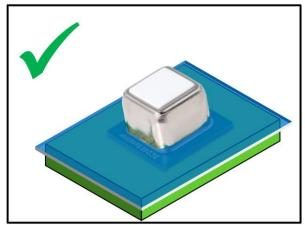
If conformal coating is applied, the top surface of the sensor (protection membrane) must remain free of coating.
